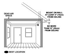
Figure 4: RECOMMENDED SMOKE ALARM MOUNTING LOCATIONS Pg. 7-3
